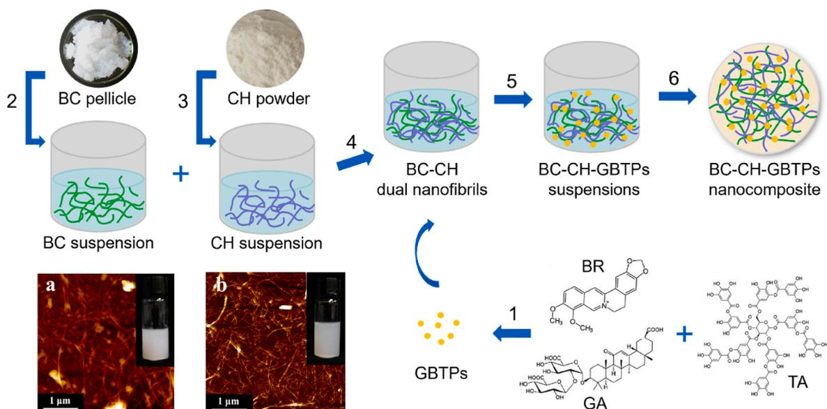
**Fig. 2.** Schematic illustration of preparation process of BC-CH-GBTPs nanocomposites. (1) Formation of GBTPs; (2 and 3) high-pressure microfluidization for preparing BC and CH nanofibrils, respectively; (4) mixing the as-synthesized suspensions of BC and CH; (5) mixing the GBTPs and suspensions of BC-CH; (6) hot-pressing at 90 °C and 0.1 MPa on a semiautomatic paper machine (Rapid-Köthen). AFM images and inset photographs of BC (a, 0.2 wt%) and CH nanofibrils (b, 0.2 wt%).
