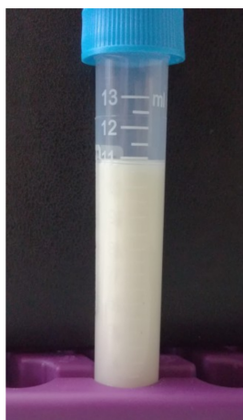
Figure 2. Optical photo of oil in water Pickering emulsion with 4 mass% of Kao in the presence of Laponite® as thickener agent.
