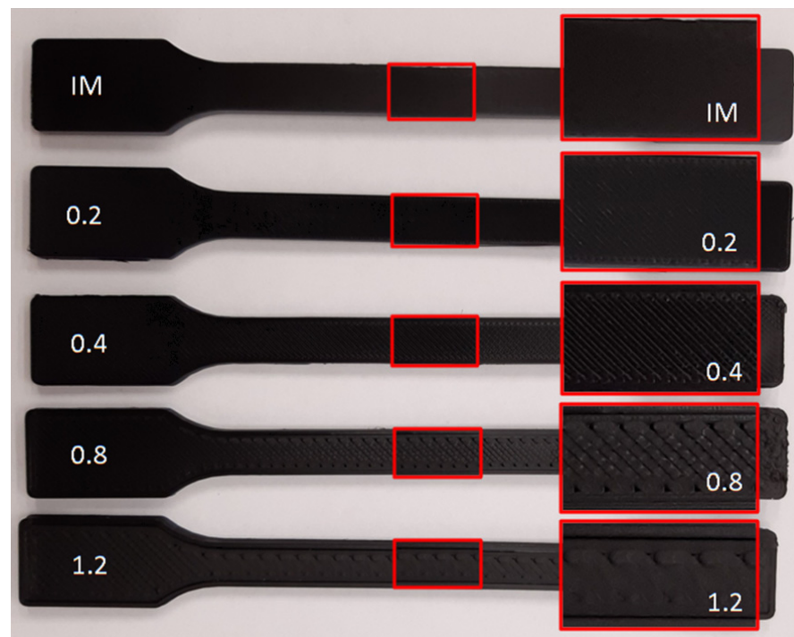
Figure 5. Filling structure of injection molding and 3D-printed samples.
