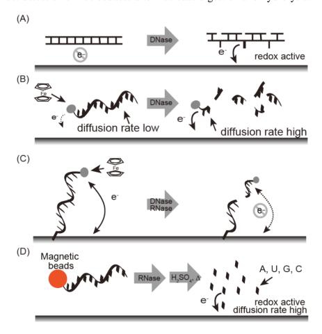
DNase can be detected by FcODN-immobilized electrodes, which provide real-time monitoring (Figure 3C). FcODN is immobilized on the electrode by Au-S linkages [23] (Figure 4A) or by reaction
