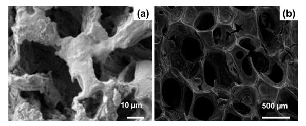
**Figure 5.** SEM images of MBG scaffolds for bone tissue engineering applications produced by porogen method (a) and replication of a polyurethane foam (b). Pictures reproduced from Yun et al. [44] and Wu et al. [40] with permission.
