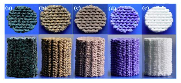
**Figure 10.** Photograph of 3D-printed scaffolds doped with different therapeutic elements: 5% Cu (a), 5% Fe (b), 5% Mn (c), 5% Co(d) and parent glass (e). Different colors were imparted to scaffolds by different dopants. Pictures reproduced from Liu et al. [97] with permission.
