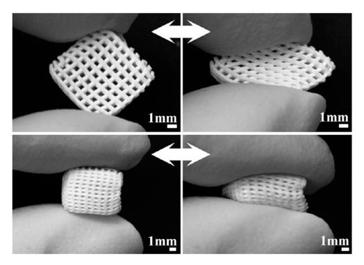
**Figure 9.** Compressibility of MBG/ polycaprolactone (PCL) composite scaffolds produced by robocasting. Pictures reproduced from Yun et al. [81] with permission.
