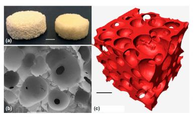
**Figure 4.** Sol-gel BG foam scaffold: (**a**) photographs after sintering at 600 °C (left) and 800 °C (right), scale bar = 5 mm; (**b**) Scanning electron microscope (SEM) image of a fracture surface, scale bar = 500  $\mu$ m; (**c**) X-ray microtomographic reconstruction of the scaffold, scale bar = 500  $\mu$ m. Pictures reproduced from Poologasundarampillai [49] with permission.
