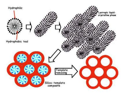
**Figure 1.** Schematic illustration of the steps leading to a mesoporous silicate material starting from a micellar solution: micelles from structure directing agent (SDA) link the hydrolyzed silica precursors through the hydrophilic component and self-assembly to form an ordered mesophase. Pictures reproduced from Arcos and Vallet-Regi [16] with permission.
