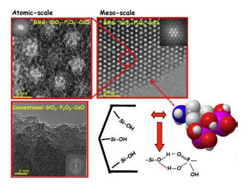
**Figure 2.** High-resolution transmission electron microscope (TEM) images of a silicate SDA-templated glass (MBG) (top) and a "conventional" sol-gel glass (without SDA) (bottom). Mesopores in the mesoporous bioactive glass (MBG) are well ordered according to a hexagonal symmetry. A schematic representation of alendronate molecule and its interaction with silanol groups at the mesopore surface are also displayed. Pictures reproduced from Arcos and Vallet-Regi [16] with permission.
