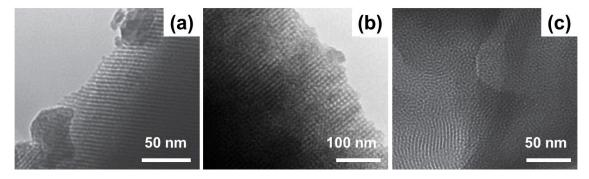
**Figure 3.** TEM images of mesoporous structures obtained by using P123 (a), F-127 (b) and cetyltrimethyl ammonium bromide (CTAB) (c) as SDAs in MBGs. Pictures reproduced from Wu et al. [33] and Yun et al. [44] with permission.
