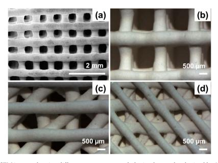
**Figure 8.** SEM images showing different macropore morphologies that can be obtained by 3D printing of MBGs: (a) squared, (b) rectangular and (c,d) irregular (triangular pattern) macropores. The high regularity of the pattern is well appreciable and macropore size is characterized by a narrow distribution. Pictures reproduced from Zhang et al. [77] and Wu et al. [75] with permission.
