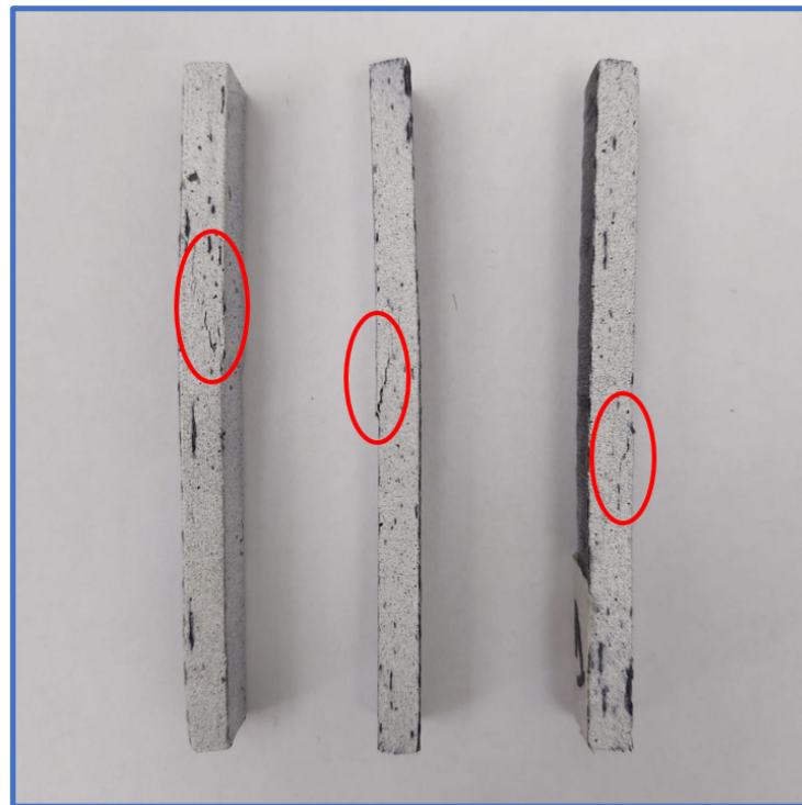
Figure 14. Bending test specimens after testing.
