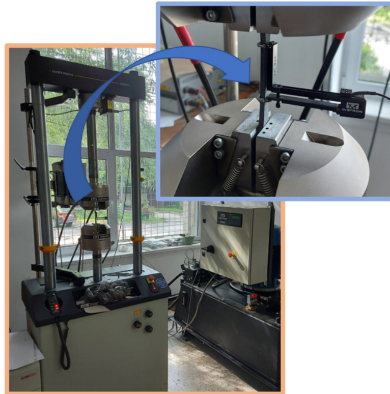
Figure 4. Tensile testing of multi-ply CFRP.
