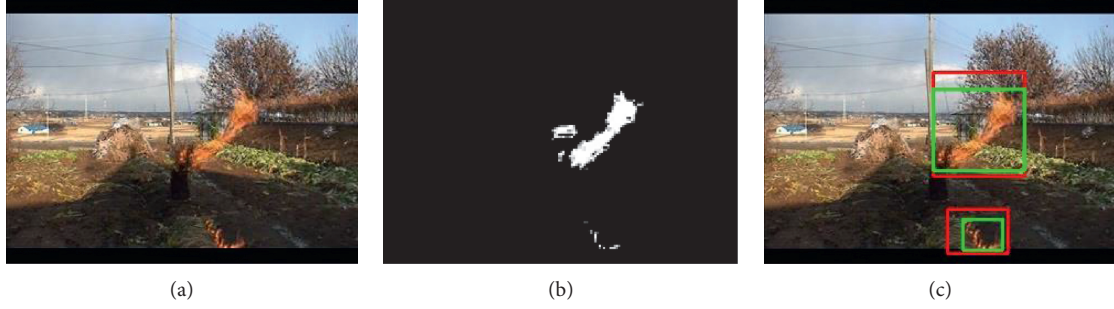
FIGURE 5: Comparison of flame color detection results and motion detection results. (b) A binary image after color detection. The red box in (c) represents the area after motion detection, and the green box represents the area after color detection. After color detection, the obtained area is more accurate.
