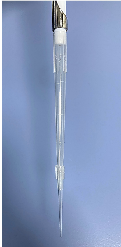
Figure 4. Double plastic tip to enhance MMS dissociation
