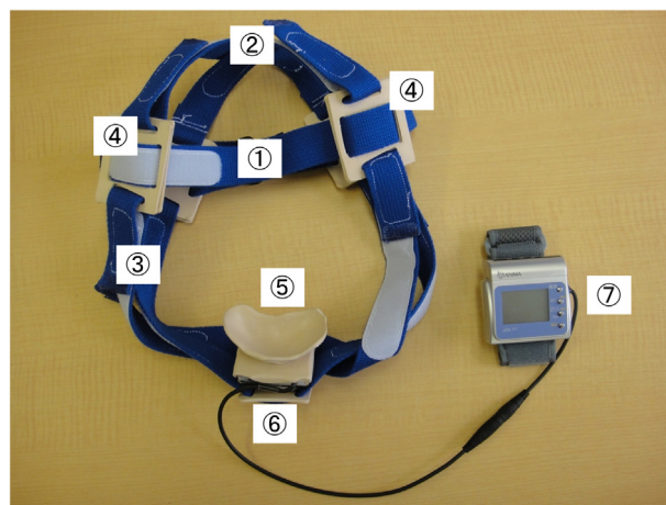
Figure 1 Jaw-opening sthenometer. The jaw-opening sthenometer consists of fabric belts, hook and loop fasteners, thermoplastic splint material (LMB Blend), and a mini-isometric dynamometer ( \mu Tas F1). (1) One head-encircling belt. (2) Two belts to secure the top of the head to the head-encircling belt. (3) Two belts to secure the mandible to the head-encircling belt. (4) Thermoplastic splint material to secure the belts, (5) Chin cap. (6) Dynamometer. (7) Monitor.
