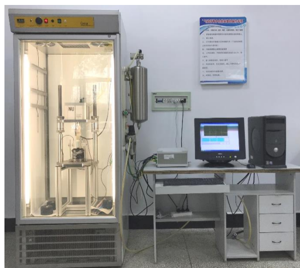
Figure 5. Uniaxial static compression creep test in this paper.
