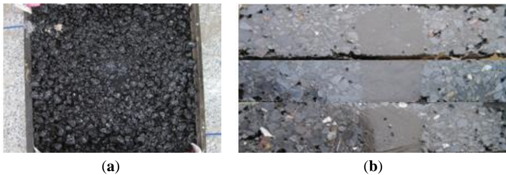
Figure 5. Cross-section of a wheel rutting test sample with the sensor embedded. (a) Wheel rutting test sample with optical fiber embedded; (b) Cross section of the test sample.
