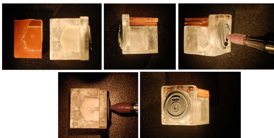
Figure 1 Aerial view of the groover with lid removed (upper left), front view of the groover (middle left), side view of the groover with the handpiece in (upper right), aerial view of the groover with the handpiece in (lower left), and side view of the groover (lower right). The interior of the chamber measures 16 mm in width, 16 mm in length (from the front to the pentagon's point, which is the back of the chamber), and 16 mm tall.
