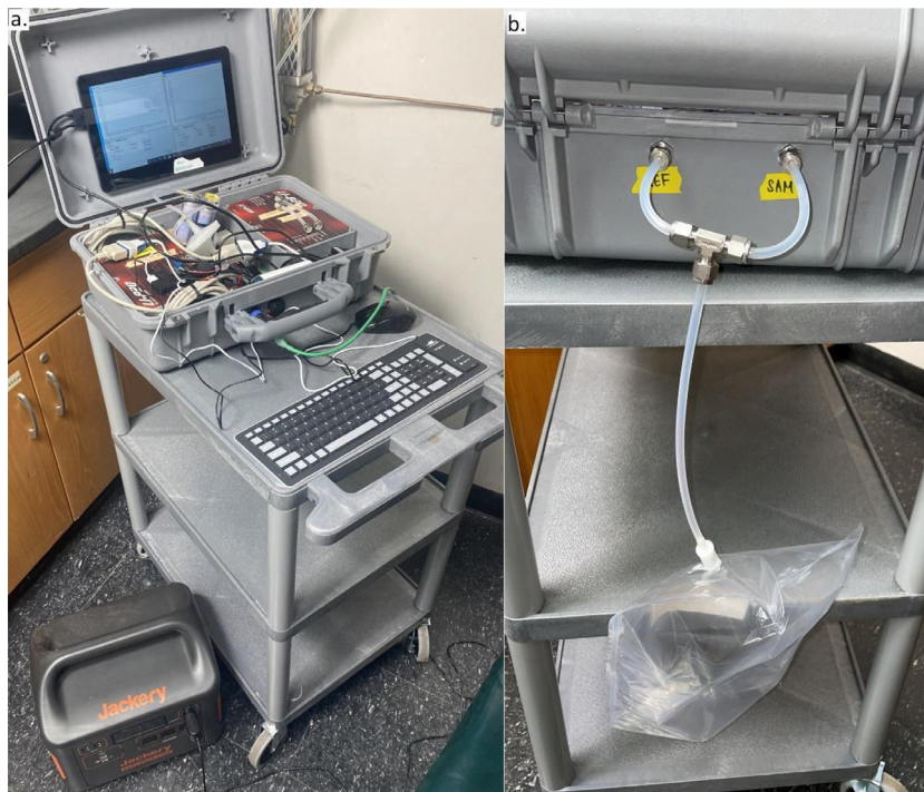
Fig. 2. Preparation of dynamic stem respiration system for its first operation in a controlled laboratory environment. a. Opening the case and switching the system on powered by a 12 VDC external battery. b. Connecting a 10 L Tedlar bag sample with 400 ppm \text{CO}_2 for calibration and match procedure prior to each 24-hour measurement period.
