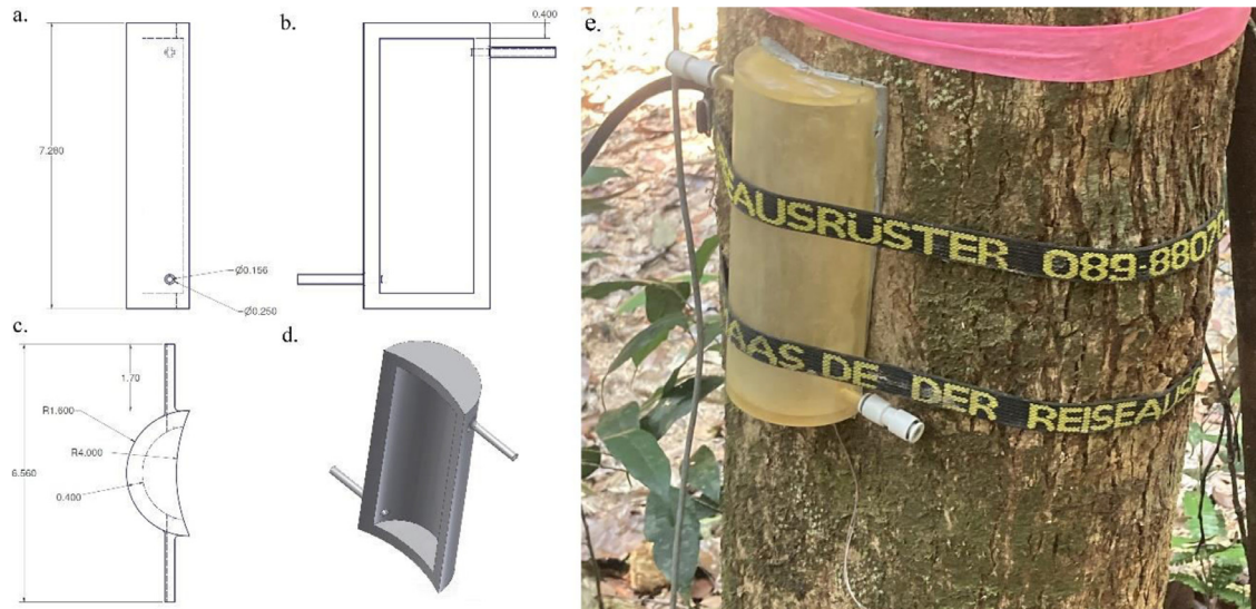
Fig. 1. Design and installation of stem chamber used for continuous observations of Es. CAD image showing a. Left, b. Back, c. Top, and d. 3D view, e. Example installation of stem chamber onto a stem using two cinch straps on a tropical tree in the Brazilian Amazon. Note the grey silicon and plastic cap above the stem enclosure used to prevent water from entering the stem chamber during rainstorms.
