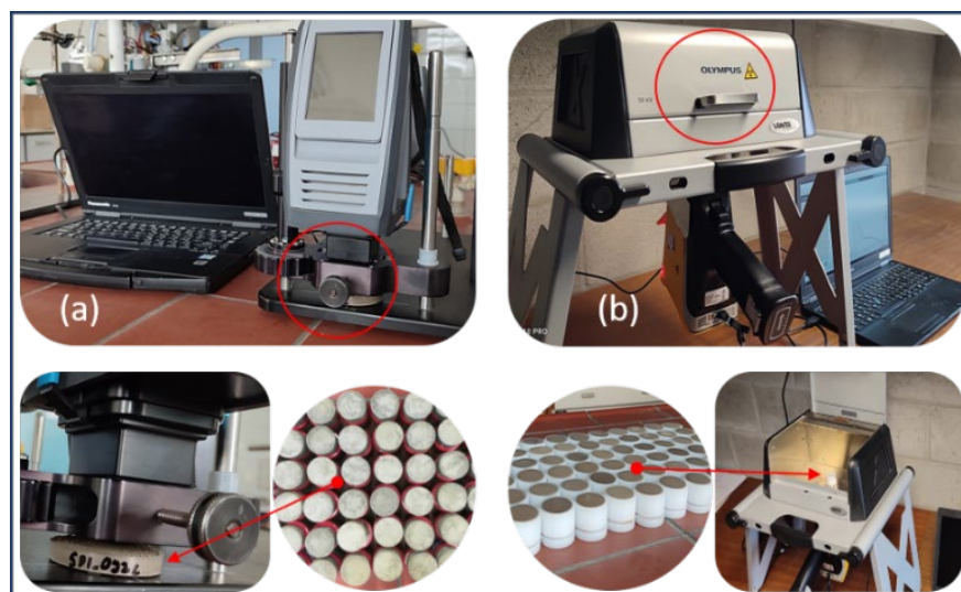
Figure 2. Experiment process for soil measurement. (a) mid infrared (MIR) scanning of soil samples, (b) X-ray fluorescence (XRF) scanning of soil samples.
