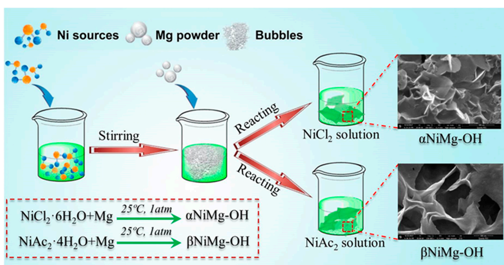
Figure 1. The diagram of the fabrication process for the \alpha -NiMg-OH nanosheets.
