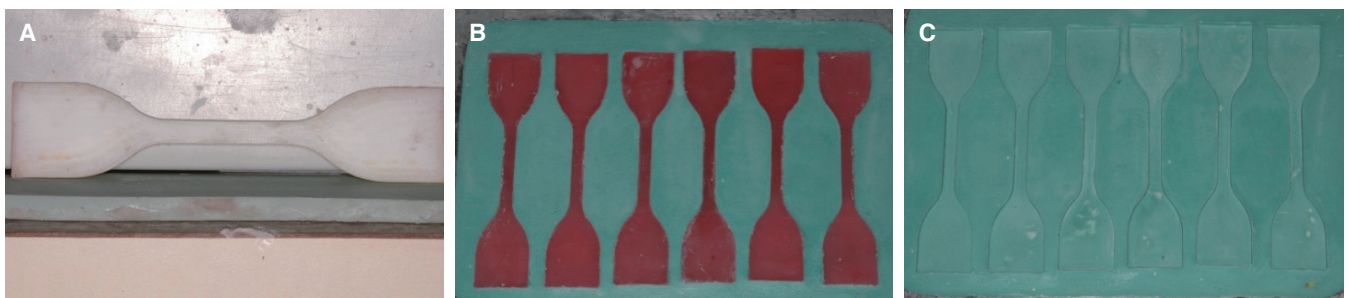
Fig. 1. (A) Master model and embedded wax patterns in flask before and after boil-out, (B) Master model and embedded wax patterns in flask before and after boil-out, (C) Master model and embedded wax patterns in flask before and after boil-out.
