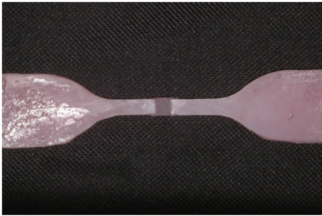
Fig. 2. Dumb-bell shaped test specimen reattached with silicone soft liner.
