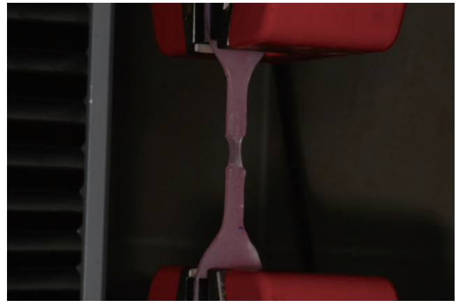
Fig. 3. Tensile testing procedure of test specimens.
