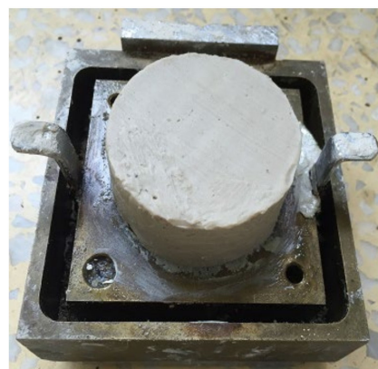
Figure 1. Standard cylinder sample of deep-sea simulant sediment.
