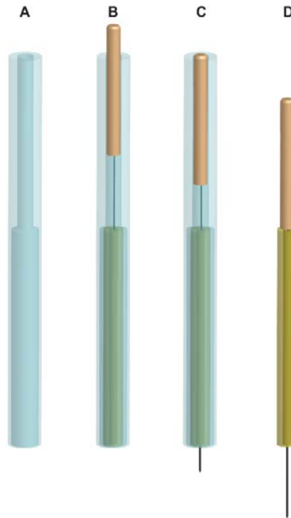
Figure 1. Penetrating needle for double blinding with outer guide tube. (A) Outer guide tube; (B) Before tapping-in method. The upper part of the needle handle protrudes from the outer guide tube by 4 mm. The inner diameter of the upper part of the outer guide tube from the top of the inner tube is slightly larger than the diameter of the needle handle, and the inner diameter of the rest of the lower part of the outer guide tube is slightly larger than the outer diameter of the inner opaque tube, which stabilizes the needle handle in the outer guide tube during the tapping-in method application; (C) After tapping-in method. The protruding part (4 mm) of the needle handle is inserted into the outer guide tube using the tapping-in method to penetrate the skin. (For the skin-touch and the no-touch placebo needle, needle tips penetrate the lower stuff in the inner tube at this stage.); (D) Needle insertion after removal of the outer guide tube. After the tapping-in method, the outer guide tube is removed, and the needle is inserted using the alternating twirling technique. The inner diameter of the inner tube is smaller than the diameter of the needle handle so that the inner tube works as a stopper. (The blunt tip of the skin-touch needle slightly protrudes from the inner tube to touch the skin but not for the no-touch placebo needle at this stage).
