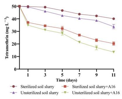
Figure 7. Degradation kinetics of tetramethrin in different soil slurries.
