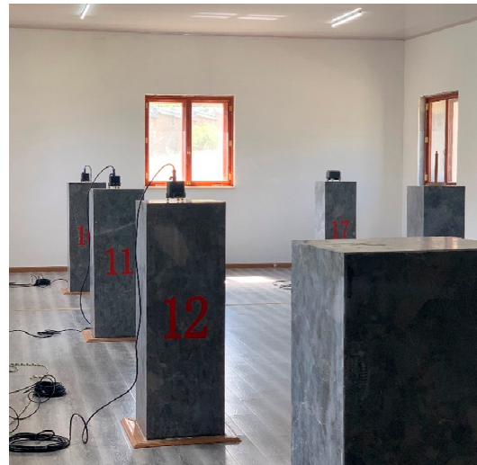
Figure 12. Photo of the observation experiment used for the fluxgate sensor comparison.
