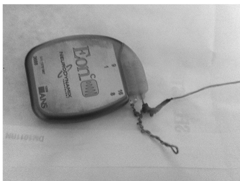
Fig. 3 IPG with twisted wires after removal from patient
