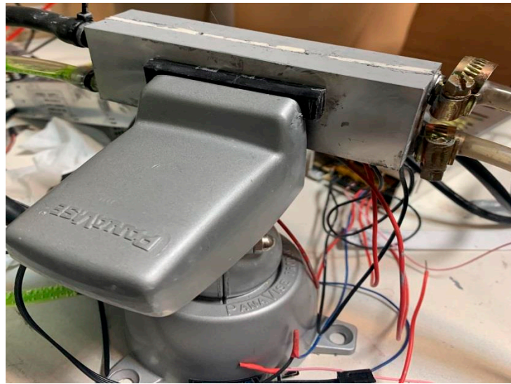
Figure 3. The aluminum block is attached to the thermoelectric modules from one side only.
