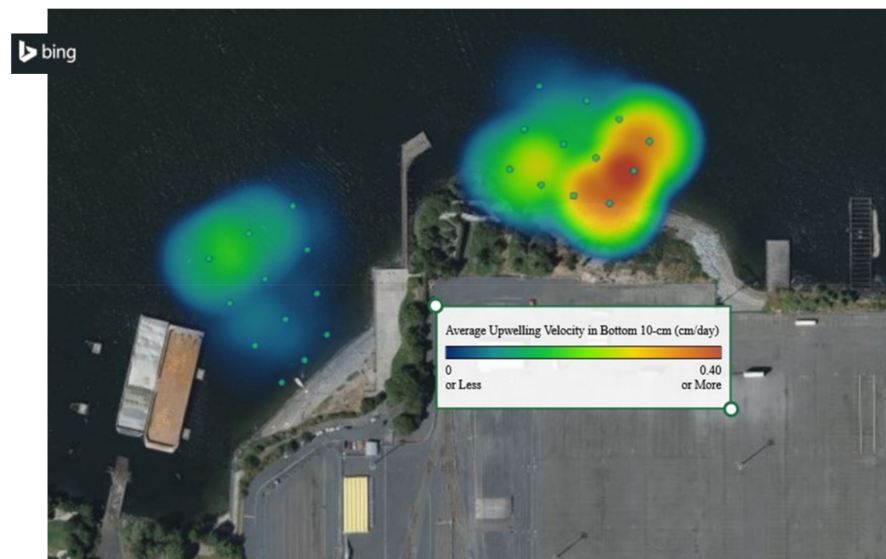
Figure 5. A heat map of the estimated distribution of upwelling groundwater flow (cm/day) averaged across the bottom 10 cm of the SPME sampler within the NW and NE sampling locations. The dots indicate the 24 SPME sampling stations. Microsoft product screen shot(s) reprinted with permission from Microsoft Corporation.
