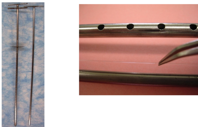
Figure 3. SPME sampler with a 90 cm working section showing perforated outer shield tube and inner rod (left). Close-up of the perforated shield tube; the inner rod with slit and the PDMS are also shown (right). The fiber has 0.59 \mu\text{L}/\text{cm} of PDMS around a 497 \mu\text{m} -diameter glass core.
