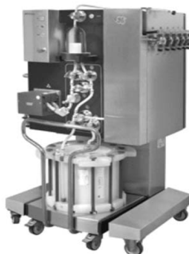
Fig. 7. Chromatographic installation AKTA™ for purifying viral suspensions on monolith columns.
