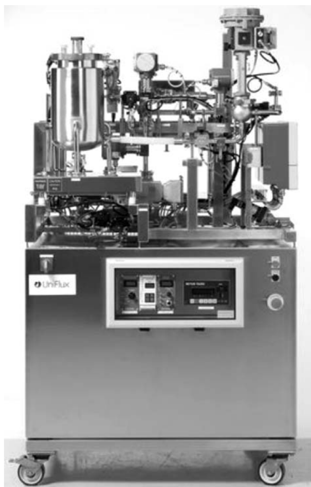
Fig. 6. The UniFlux system for the concentration of biomaterials, outer view.
