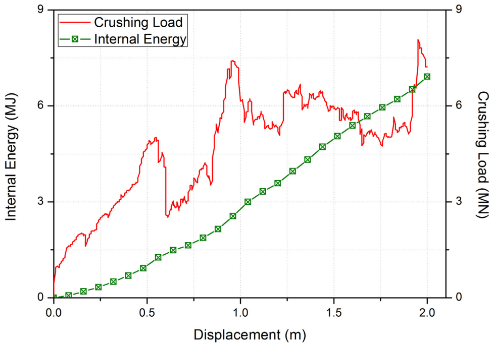
Fig. 7. Energy and load for perpendicular collision.
