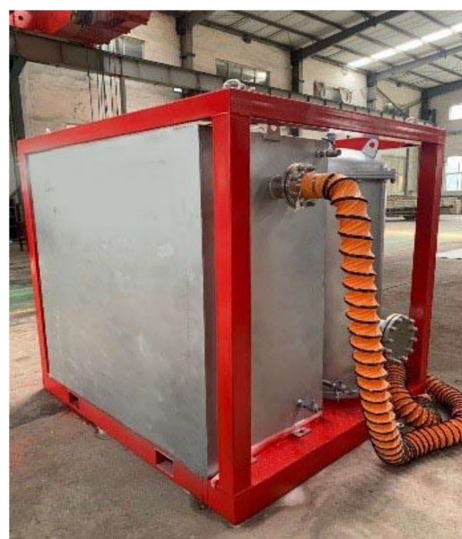
(b) Venturi-bubbling reactor (500Nm 3 /h) 1720mm*1720mm*2000mm
