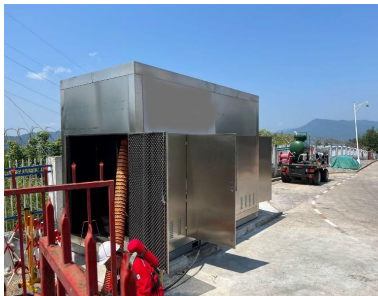
(a) Bubble reactor (1000Nm 3 /h) 4000mm*1900mm*2600mm
