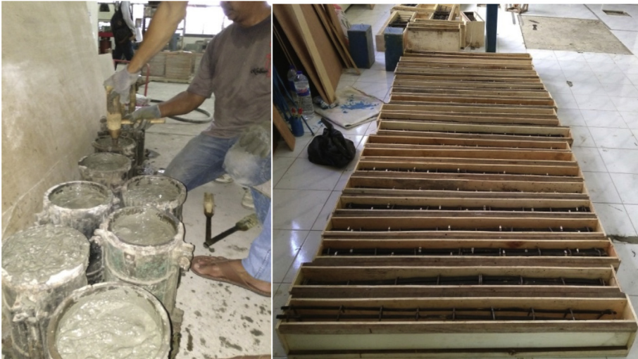
Fig. 12. Preparing pull-out test and flexural test specimens.
