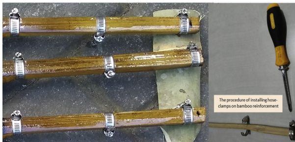
Fig. 10. The installation of hose-clamps and the second layer of Sikadur®-752 adhesive.
