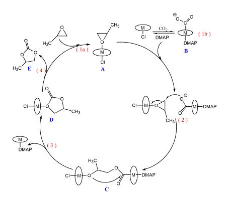
Scheme 2. Proposed mechanism for the cycloaddition of propylene oxide to CO<sub>2</sub> with DMAP.
