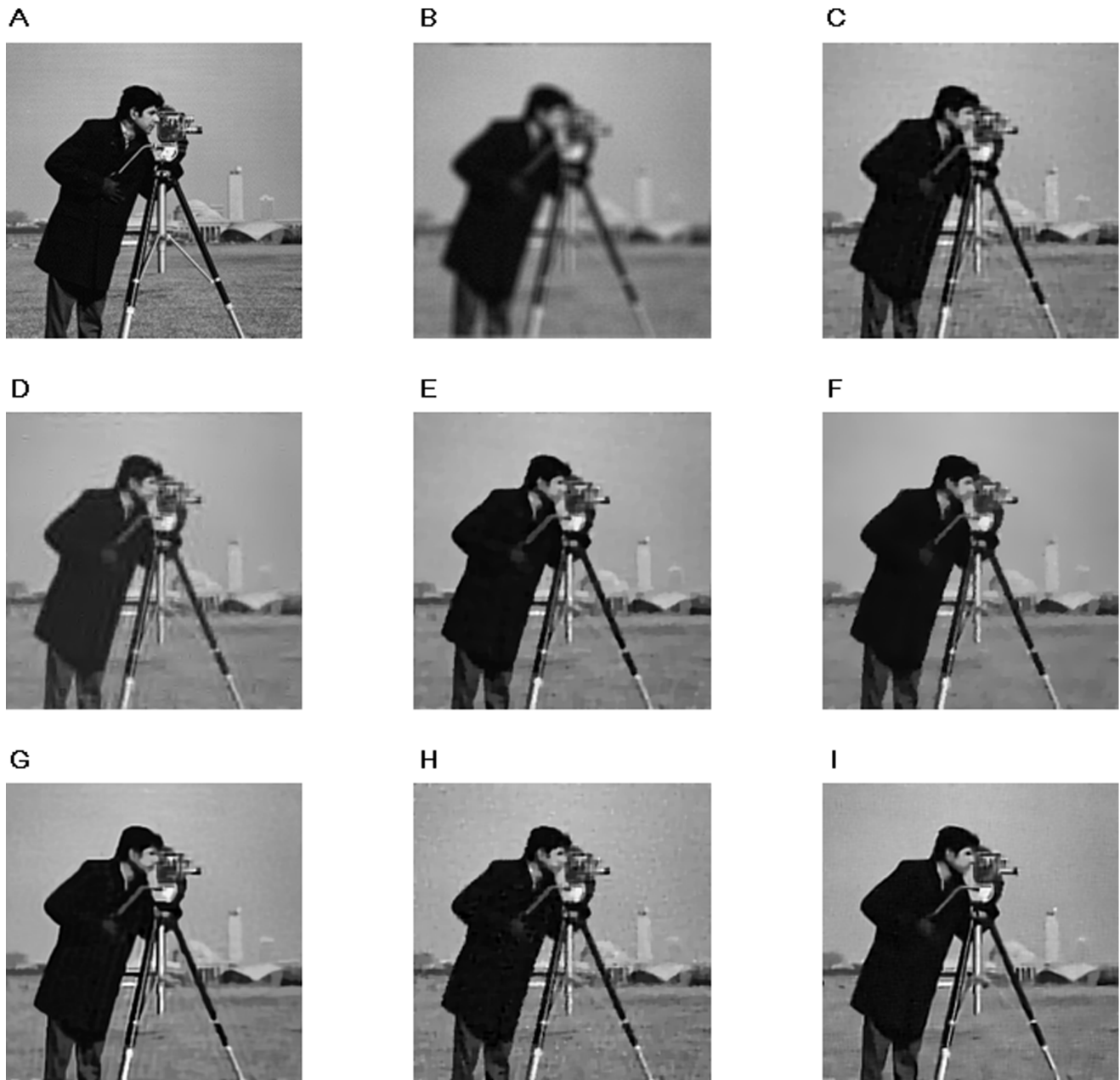
Figure 3. Restoration results on a 256 \times 256 Cameraman image degraded by a 9 \times 9 average kernel and a gaussian noise with \sigma = 2 . A. Original Image B. Degraded Image C. Operator Splitting TV D. ForWard E. FTvd F. FAST-TV G. NLTv+BOS H. Algorithm 1 I. Algorithm 2. doi:10.1371/journal.pone.0065865.g003
