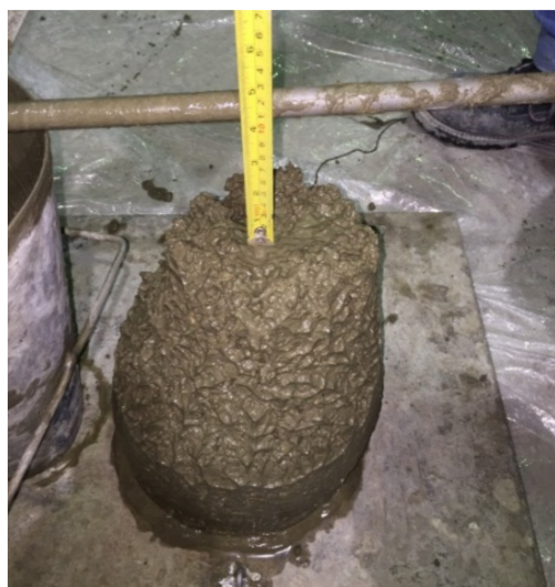
Figure 10. Slump measurement using the cone test method.
