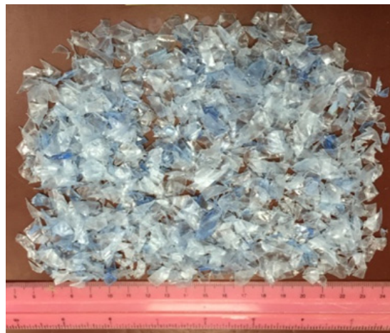
Figure 4. Polyethylene terephthalate (PET) plastics waste used in developing plastic based green lightweight aggregate (PGLA).
