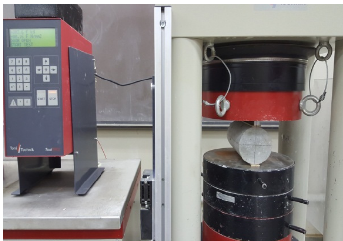
Figure 13. Test setup for splitting tensile strength test.
