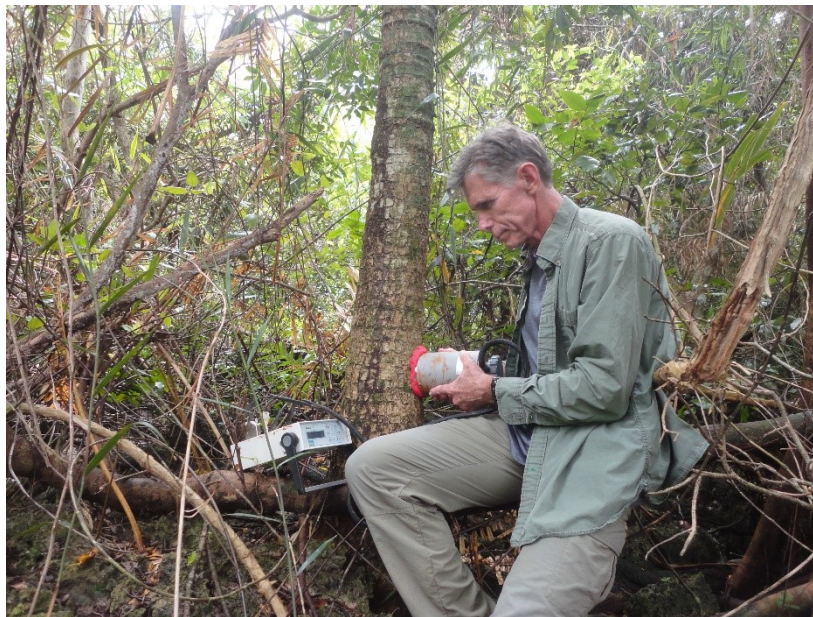
Figure 5. Depiction of the infrared gas exchange instrument (left) and chamber in use near the base of a Cycas stem with red malleable modeling clay used for seal.
