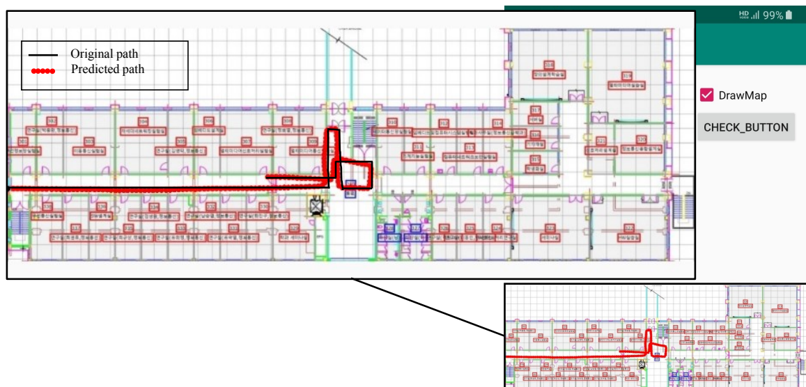
Figure 4. Direction estimation and distance estimation using the developed application for path geometry 1. The enlarged part of the screenshot shows the original and predicted paths.
