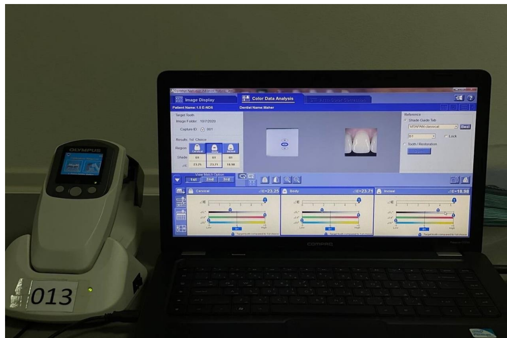
Figure 3. Shade detection of ceramic specimens using Crystaleye Olympus spectrophotometer.
