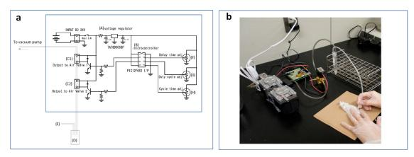
**Figure 1.** Mouse milking device. (**a**). Schematic circuit diagram of milking device. Voltage regulator (A), a microcontroller (B), two solenoid valves (C1 and C2), a milk-receiving tube (D), a teat cup (E), and three variable resistors (F, G, H). (**b**) Mouse being milked using the milking device.
