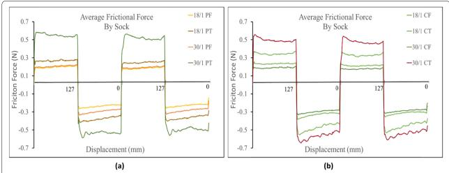
Fig. 9 (a) Comparison of spun polyester fibers based on corresponding fabric structure, yarn type and linear density against Lorica skin simulant (b) Comparison of spun cotton fibers based on corresponding fabric structure, yarn type and linear density against Lorica skin simulant
