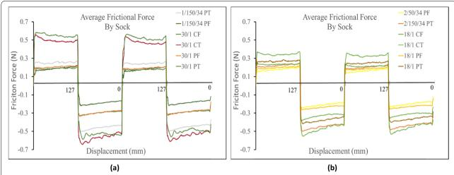
Fig. 7 a Linear density comparison of terry knit samples against Lorica skin simulant. b Linear density comparison of single jersey knit samples against Lorica skin simulant
