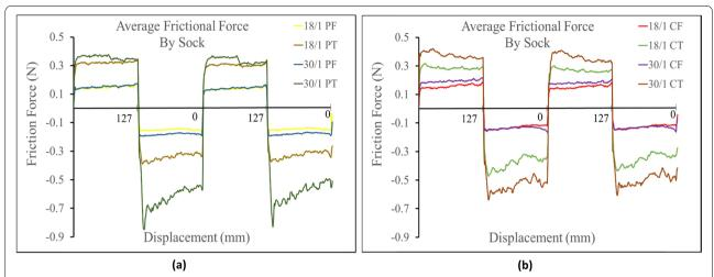
Fig. 5 (a) Comparison of polyester fiber based on corresponding fabric structure, yarn type and linear density (b) Comparison of cotton fiber based on corresponding fabric structure, yarn type and linear density
