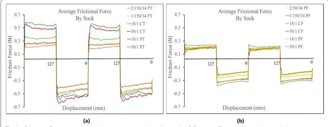
Fig. 6 a Friction profiles comparing terry knit structures against Lorica skin simulant. b Friction profiles comparing single jersey knit structures against the Lorica skin simulant
