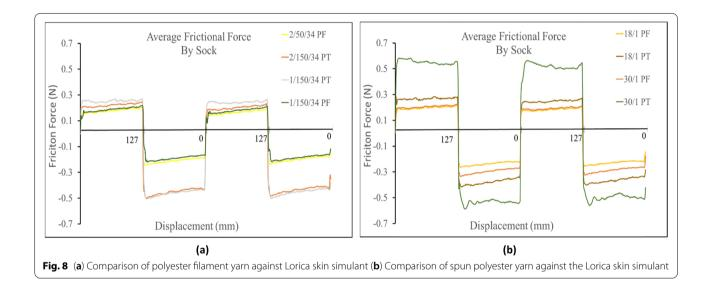
terry knit samples. From these trials the 2/150/34 terry knit samples registered a slightly higher frictional force than the 18/1 spun yarn sample. The cause of this deviation is unknown and would need to be investigated further.
