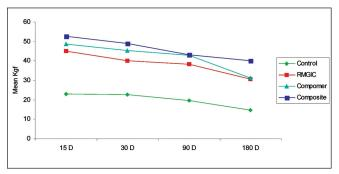
Figure 6: Load failures of various materials at determined time intervals
