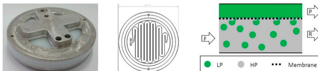
Figure 2. Miniaturized device for intensification of liquid-liquid extraction (membrane extractor). Exterior view of the device ( left ); inner channel structure ( middle ); schematic representation of the hypothesized membrane based phase separation ( right ). Feed (F), retentate (R) and permeate (P) channels are shown.
