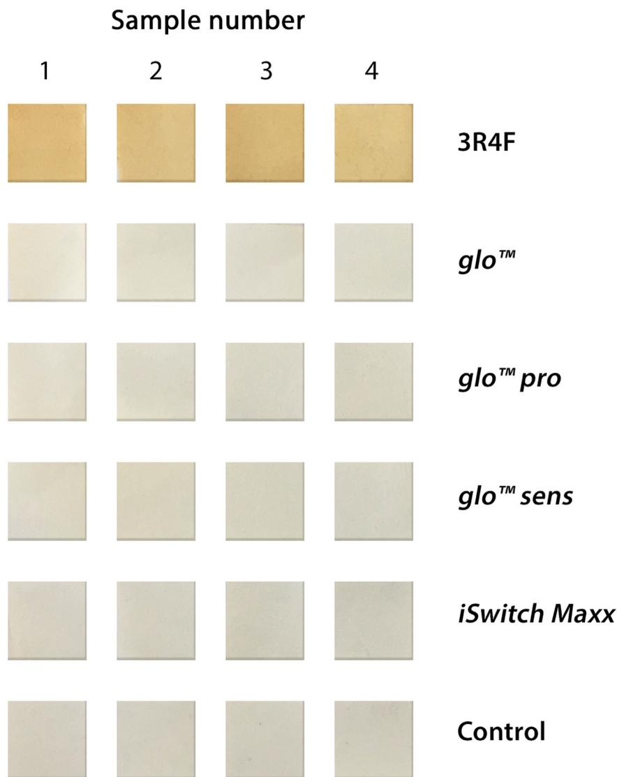
**Figure 3. Wallpaper staining following exposure to product aerosols.** Wallpaper samples were exposed to 1000 puffs of aerosols generated, from top to bottom, 3R4F CS, glo™, glo™ pro, glo™ sens and iSwitch Maxx. Control samples are unexposed samples.
