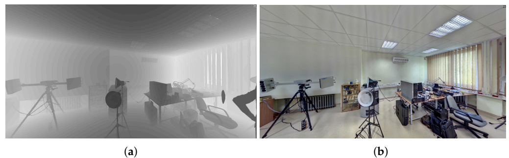
Figure 10. An indoor scene scanned by Z+F 5010C and displayed as depth map (a), darker=closer) and reflective index (b).
