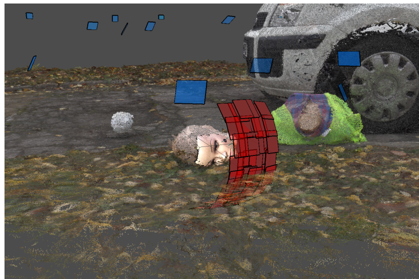
Figure 1. Fusion of short- and long-range photogrammetry.
