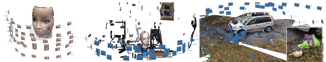
Figure 2. Photogrammetric reconstruction for close-range, middle-range, and long-range photography.
