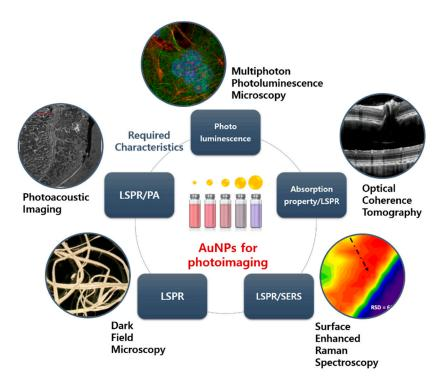
**Figure 4.** AuNP-based photoimaging. Each imaging system is arranged by required characteristics of AuNP. Image courtesy of Nikon (dark field microscopy), YSP (photoacoustic imaging (PAI)), phoenix (optical coherence tomography (OCT)), ZEISS (multiphoton photoluminescence microscopy), Sigma-Aldrich (surface enhanced Raman scattering (SERS)), respectively.
