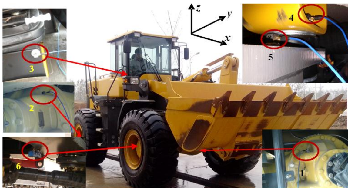
Figure 3. Vibration test site: 1—Front axle housing, 2—Rear axle housing, 3—Seat bracket, 4—Before cab mount, 5—After cab mount, 6—Front axle input shaft.
