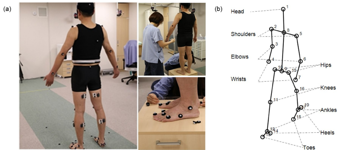
Figure 1. (a) Using Helen Hayes Marker set to capture the motion during walking trials. (b) Seventeen anatomical points were extracted from the motion capture data. Sixteen body segments (solid line) were defined by connecting the anatomical points.
