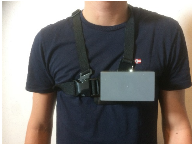
Figure 2. Ambient conditions box with temperature and humidity sensors and data receiver and storage.
