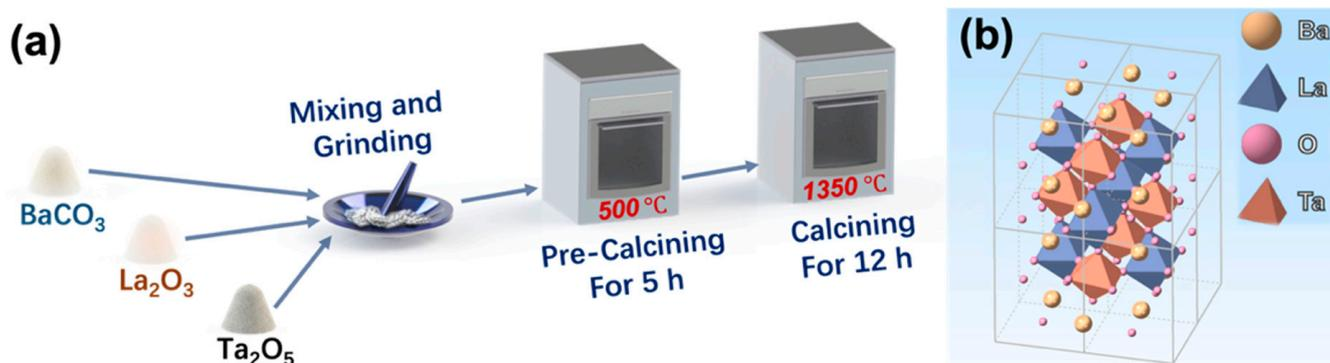
**Figure 1.** (a) Synthesis process of BLT. (b) Crystal structure schematic of BLT.
