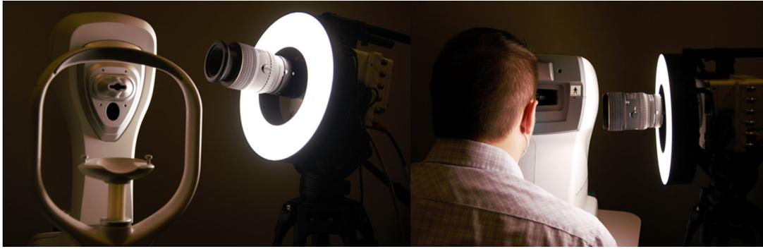
**Figure 1.** The experimental setup showing LED light mount on the camera and its location with respect to the CorVis ST and ORA devices.
