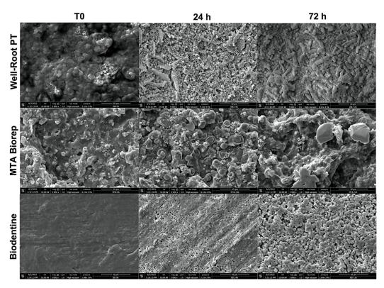
**Figure 3.** Scanning electron microscope images ( $5000 \times$  magnification) demonstrate the morphological changes of each material at 24 and 72 h of immersion in phosphate-buffered solution at 37 °C.
