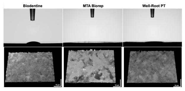
Figure 5. Contact angles of 5  $\mu$ L of water drop on the different cement surfaces after 10 s. Digital micrographs of the different surfaces using KEYENCE 7000 VHX demonstrate the roughness of each material.
