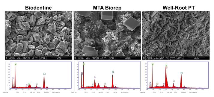
**Figure 4.** Scanning electron microscope images ( $5000 \times$  magnification) demonstrate the morphological changes and EDX spectrums of each material at 168 h of immersion in phosphate-buffered solution at 37 °C.
