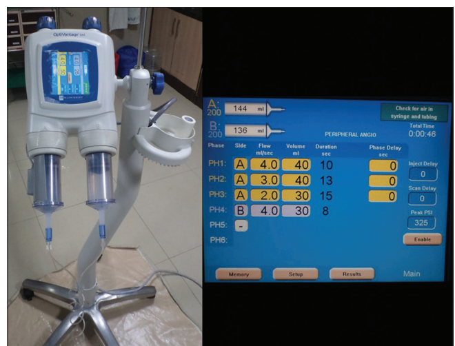
Figure 5 (A-C): CT Pressure Injectors: (Covidien CT OptiVantage DH) Functional issues in newer CT pressure injectors include (A) programmable user defined protocols (B) colour pressure sensitive touchscreen that offers different colours for operations like loading, arming, injecting (C) availability of vendor specific sensors such as RFID-enabled syringes/power injectors, and syringe volume sensors
