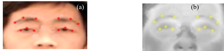
Figure 9. Landmarks as control points for registration accuracy evaluation: (a) visible image; (b) IR image.
