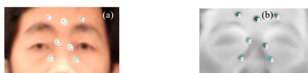
Figure 7. Aluminum Markers as control points for registration accuracy evaluation: (a) visible image; (b) IR image [19].
