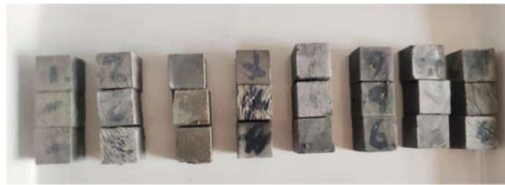
Figure 3. Cement slurry test block.
