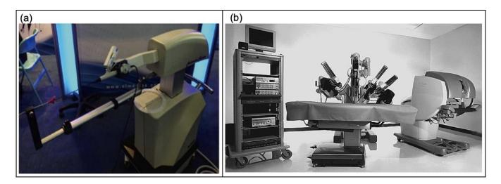
**Figure 13.** Robotic surgery instruments. (a) The robotic flexible ureteroscopy machine [54]. (b) The da Vinci surgical system. From left to right: image processing stack, a patient-side cart containing robotic arms and the surgeon's console [138]. Copyright 2007, IEEE.
