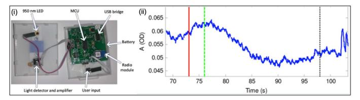
**Figure 4.** Near-infrared spectroscopy method. (i) NIRS device used for monitoring urine in the bladder; (ii) attenuation detection during voiding. The red, green and black lines are permission to void, beginning and end of voiding, respectively [87]. Copyright 2014, IEEE.
