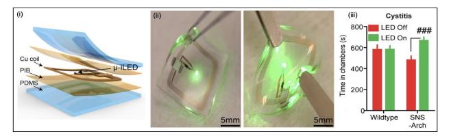
**Figure 15.** Optoelectrical system for interstitial cystitis. (i) Schematic depiction of the layered optoelectronic device, (ii) demonstrating the flexibility of the device using forceps, and (iii) a graph showing that SNS-Arch mice display a significant response for LED ON compared to LED OFF, whereas wild-type mice have no preference (### p = 0.0065, 11 mice per group, two-way analysis of variance (ANOVA)) [45].
